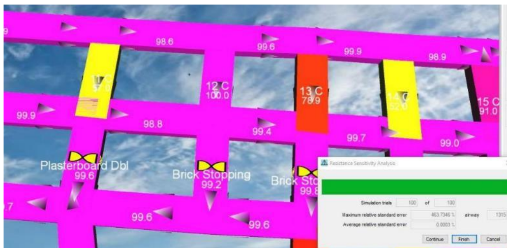
Figure 29-29-1 Results after completion of the resistance sensitivity analysis, showing the Confidence Quantity (%). Low confidence in the airflow quantity is often found in cross-cut airways,
