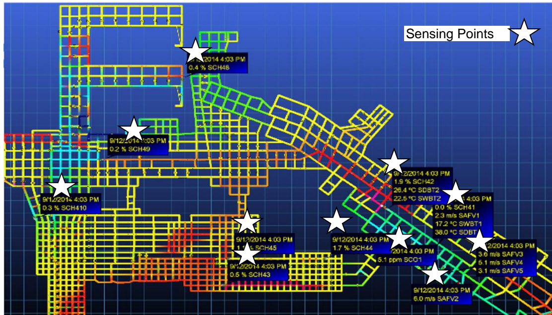
Figure 4: Transient Simulation of Downstream Sensors Gases (gas concentrations shown in different colours)
