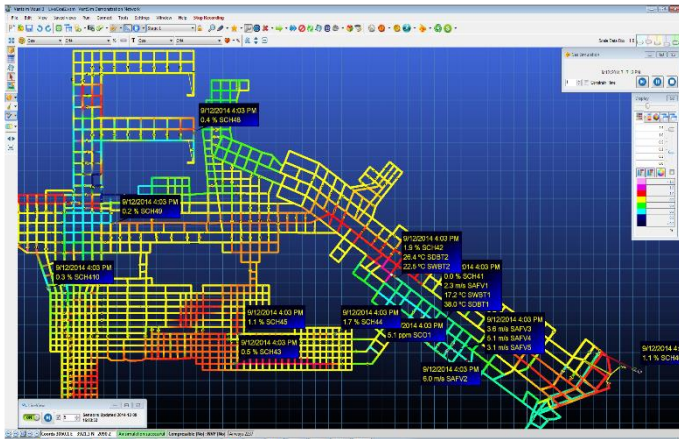
Figure 6 Mine Ventilation Modelled from Sensor Data
