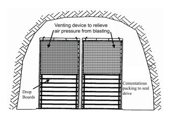
FIG 2 - Possible venting device or arrangement for regulators.
