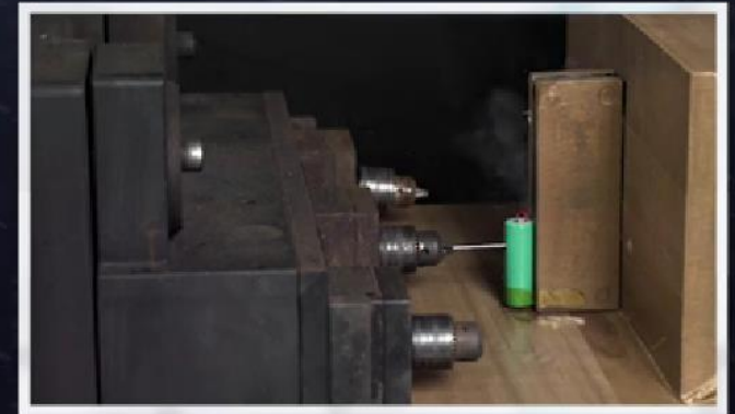
Normal LiFePO4 Lithium Iron Phosphate Battery: Battery liquid leaks, smoke observed, surface temperature exceeding 110°C
