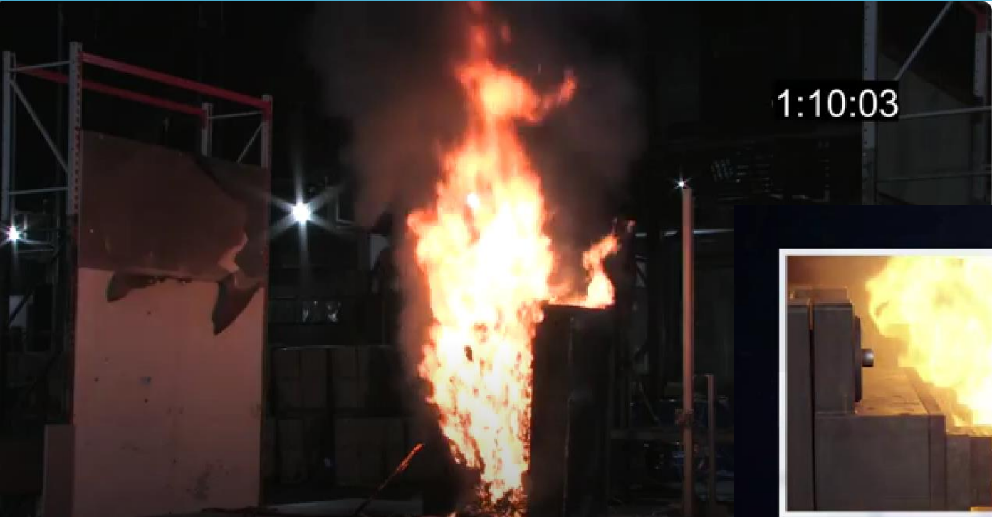
Li-NMC Lithium Battery: Severe burning surface temperature exceeding 500°C
