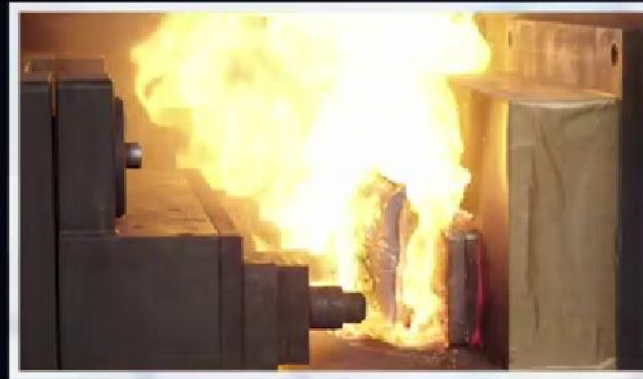
Li-NMC Lithium Battery: Severe burning surface temperature exceeding 500°C
