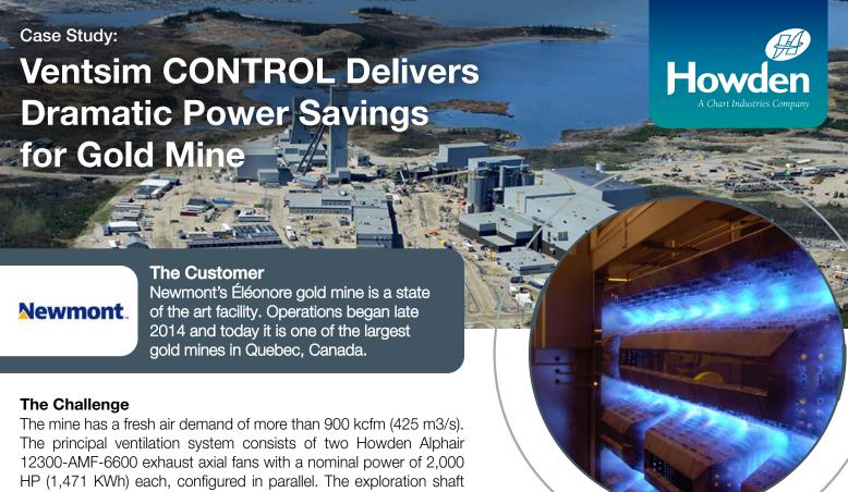
has two Howden Alphair 11200-AMF-6600 main intake fans with a nominal power of 750 HP (551.62 KWh), again configured in parallel. Lastly, there are over 140 underground auxiliary and booster fans operated in conjunction with seven dampers and air regulators, and a propane fuelled heating system. The challenge was to provide an overarching automated control system maximising safety and ventilation efficiency, whilst reducing energy demands and costs.
